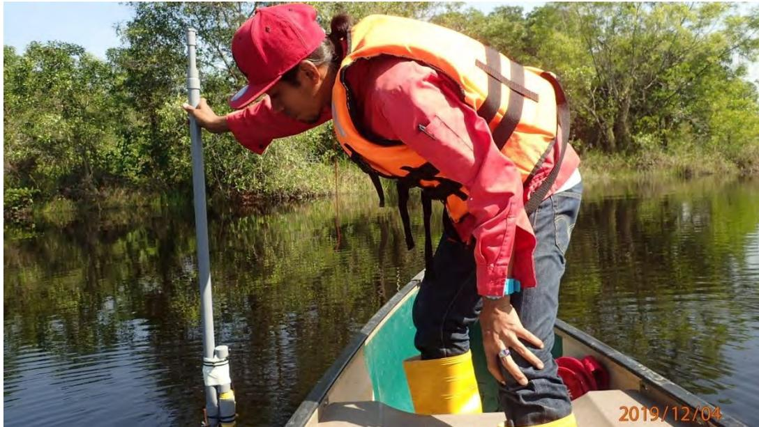
Plate 2-5: A depth sounder being used on a lake at Paya Indah Wetlands
