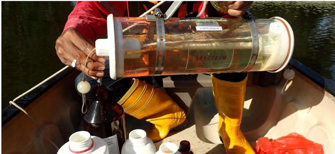
**Plate 2-6: A Van Dorn Sampler being used for lake water sampling**
