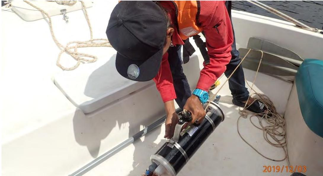
**Plate 2-8: Lab assistant with lake water sample in a Van Dorn sampler**
